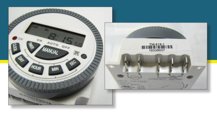
The TM620 is a 7 day timer that allows up to 6 on/off functions per day with times down to ONE SECOND. It is available in 120VAC. First, please check that you have the correct voltage for the application. The specified voltage is for the timer only. The output to your timed device goes through the contacts of the output relay which is rated to a maximum of 16A resistive and 8A inductive at 250VAC, 20 amps resistive at 125VAC and 16A at 30VDC.
